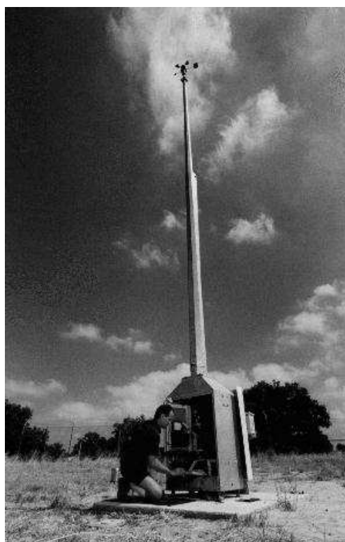
Figure 2: Typical automatic weather station (AWS).
